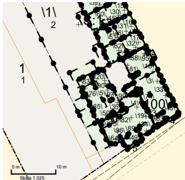
Figure 4. Selection from cadastral index map used in the City of Stockholm, showing around 50 of the close to one thousand 3D property units registered within the Stockholm municipality. City of Stockholm 2023
