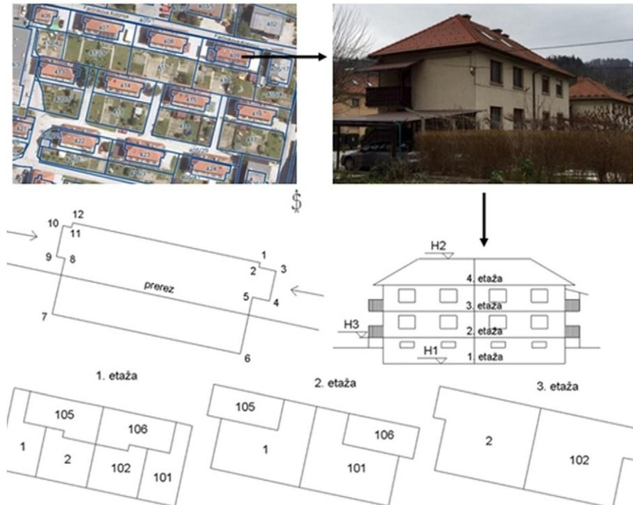
Fig. 10. A land cadastre map with land parcels and buildings' footprints on orthophoto (upper left corner), and graphical representation of the selected building in the building cadastre (the projection of the building to the ground, vertical section with characteristic heights, and floor plans).
