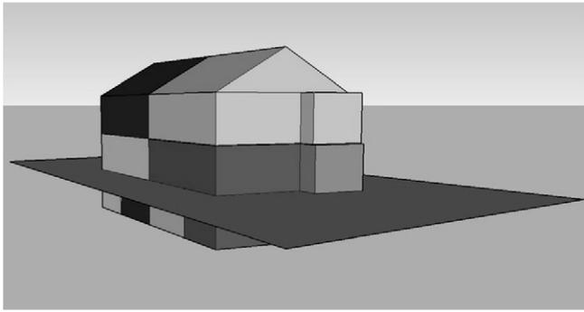
**Fig. 11.** 3D model of the selected building based on cadastral and additionally acquired data (floor heights).
