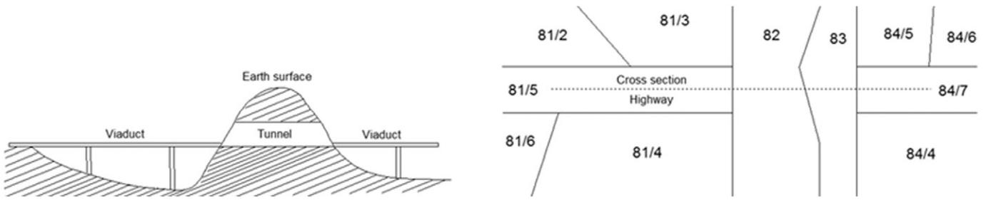
Fig. 9. The third case study: real situation – proposed 3D model (left); current cadastral representation (right).
