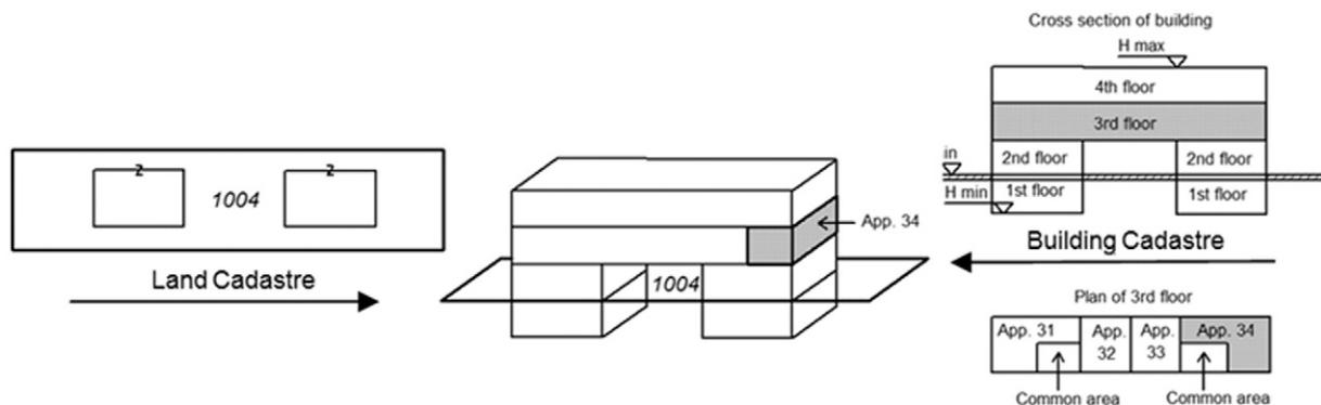
Fig. 8. The second case study: land parcel boundaries and footprints of the building in the land cadastre (left), the proposed 3D representation of real property (in the middle), and data recorded in the building cadastre (left).
