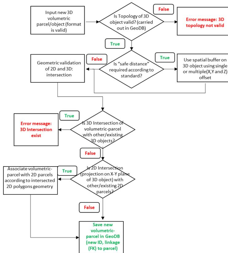
Figure 2. An example of a cadastral process: Insertion of a new 3D object workflow.
