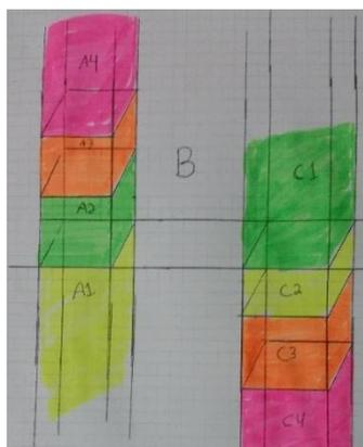
Figure 1. A, B, C are 2D parcels. A1, A2, A3, and A4 are 3D volumetric parcels in the 'air column' of A. C1, C2, C3, and C4 are the 3D volumetric parcels in the 'air column' of C.
