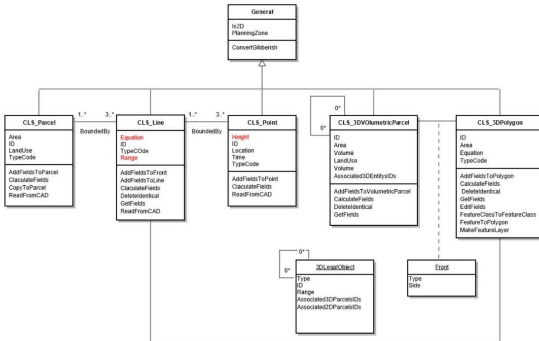
Figure 5. Main classes in SOI's operative cadastral system; integrated with new classes that should be added to the cadastral system to serve the 3D reality. Fields in red are relevant only for 3D representation.
