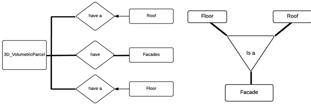
Figure 7. Left: A 3D\_VolumetricParcel must have a Roof, Facades, and Floor. Every Floor and Roof belongs to a 3D volumetric parcel. Right: Floor and Roof are Facades in a different orientation.
