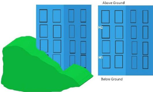
Figure 4. Levels with the same orthometric heights (absolute height) could be either above or below ground (relative height).
