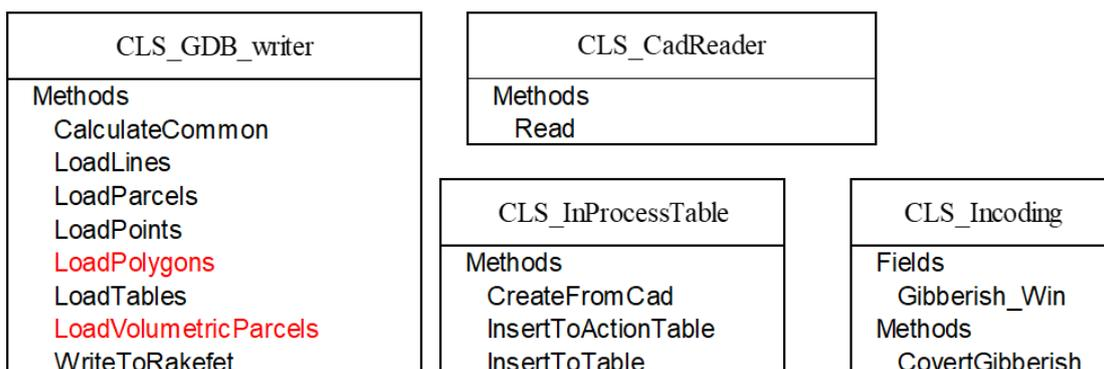
Figure 6. Classes used for reading the input data from CAD files and writing them into the geo-database and tables.
