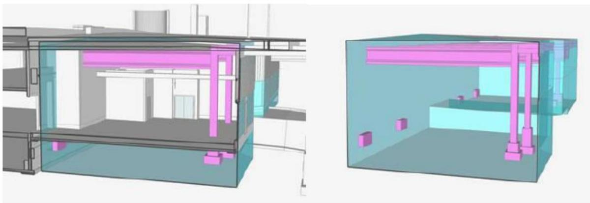
**Figure 6.3. Left: 3D property boundaries (in turquoise colour) and property rights (pink colour) and internal construction details (Andrée et al., 2018b, p. 46). Right: 3D property boundaries (in turquoise colour) and property rights (pink colour) without internal construction details (Andrée et al., 2018b, p. 46)**
