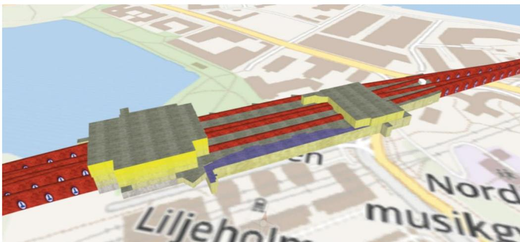
**Figure 11. 3D property formation of subway station in Stockholm (Source: <http://www.sl4d.se/pilotprojekt-3.html>)**
