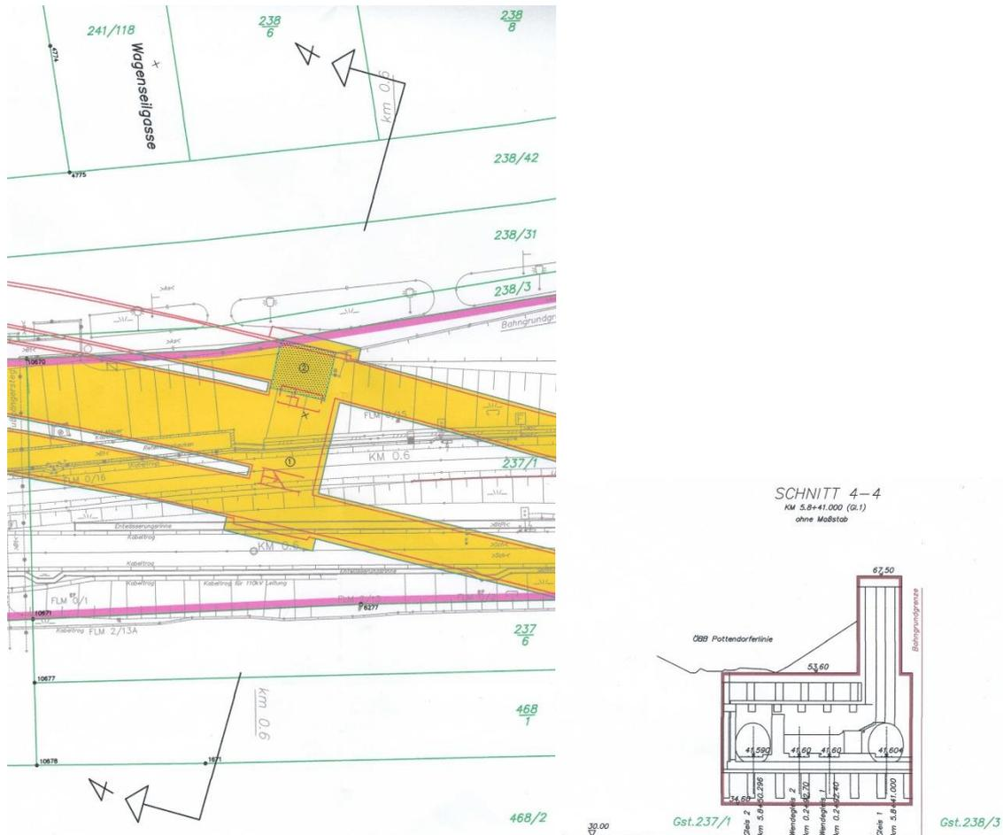
**Figure 2. Details from easement plan for the subway line U6 (data: Korschineck & Partner Vermessung ZT-GmbH)**
