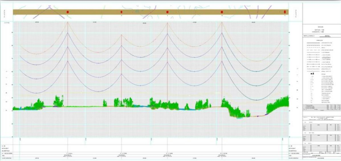
**Figure 11. Profile of the terrain generated from LiDAR data integrated with the electrical project**
