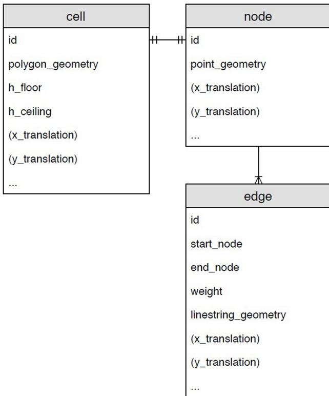
Fig. 9. The basic concept of 2D database storage.
