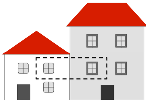
Figure 2. Example of a complex 3D cadastre case not detectable at street level: a single apartment shared by two different buildings (de Almeida et al, 2014)
