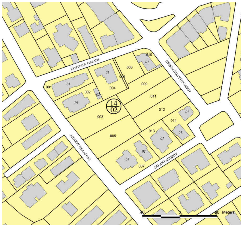
Typical cadastral map showing land parcels and buildings in an urban area in Greece
