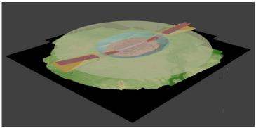
Figure 4. 3D eTOD Obstruction Identification Surfaces in 3D pdf (Source: http://gis.icao.int/ETOD/tod.pdf)
