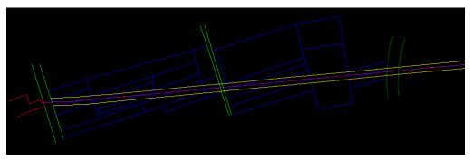
Figure 9. Cadastral survey plan of power line (down) presentation of 3D restrictions due to servitude of passage (servitude is coloured in yellow, powerline centre line in purple, land parcel borders in blue and roads in green)
