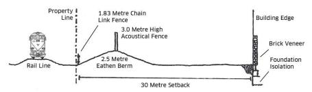
Figure 5. Mitigation measures for developments in the proximity of railway (Source: Guidelines for New Development in Proximity to Railway Operations, 2013)
