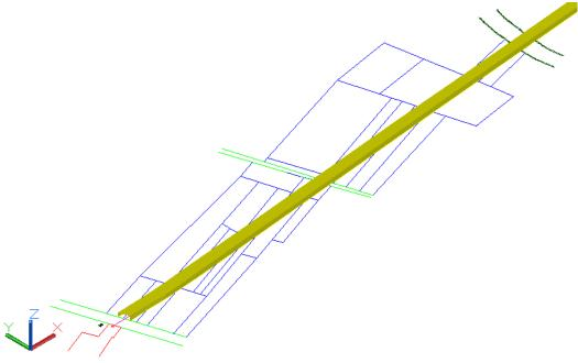
Figure 10. Presentation of 3D restrictions due to servitude of passage (servitude is coloured in yellow, powerline centre line in purple, land parcel borders in blue and roads in green)
