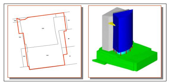
Figure 6. Examination of spatial conditions of an underground parking (depicted in green in the right picture), and 2D parcels (depicted in black in the left picture). Intersection output will produce partial intersection (source: The SOI)
