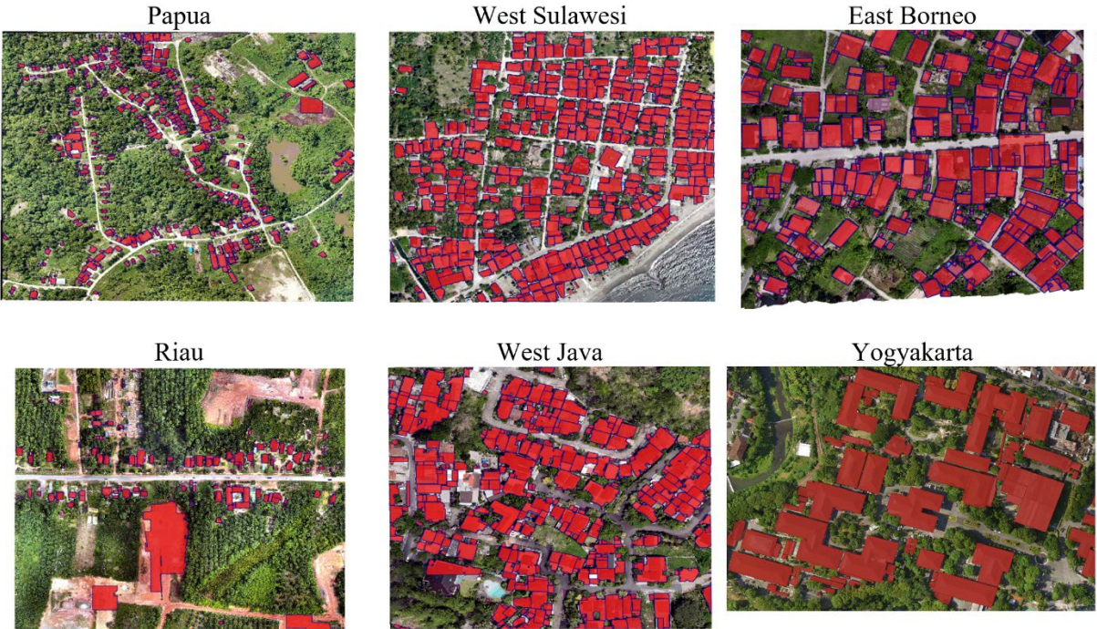
Figure 12. The resulting building footprint by YOLO deep learning with a custom trained model
