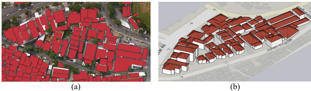
Figure 3. AI result for building detection (a) and sample result of 3D building modeling (b)
