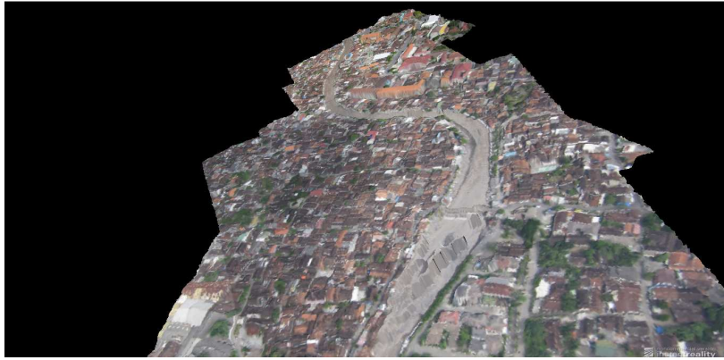
Figure 9. Topographic data acquired from aerial photography converted to X3D format
