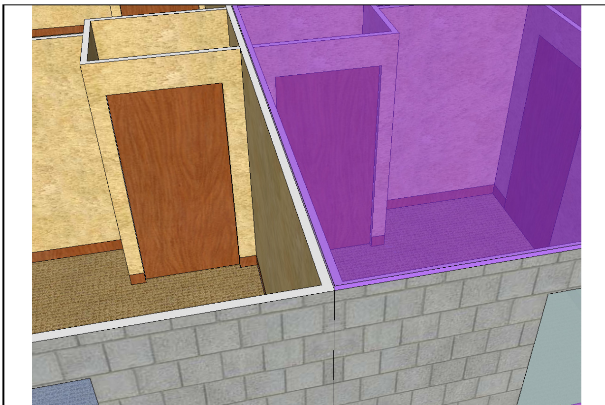
Median face: The ownership boundary right is defined as median face for the purple lot. Therefore, half of the wall belongs to the purple lot.
