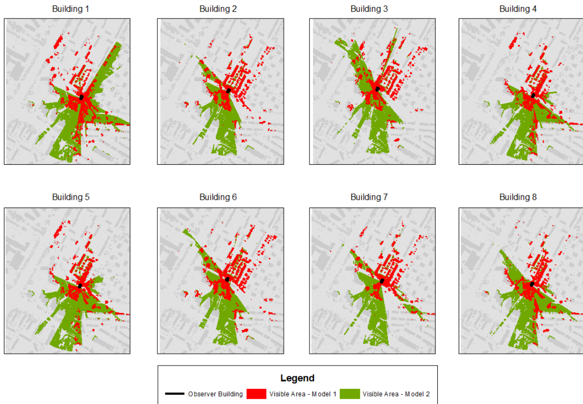
Figure 9. Comparison of visible area with 'Model 1' and 'Model 2'
