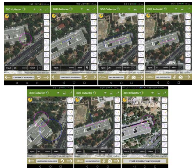
Figure 5. Geometrical drawing tools offered by BoundGeometry application. Top (left to right): circle, line, offset to line, vertical lines Bottom: intersection points between 2 circles, 2 lines, a circle and a line
