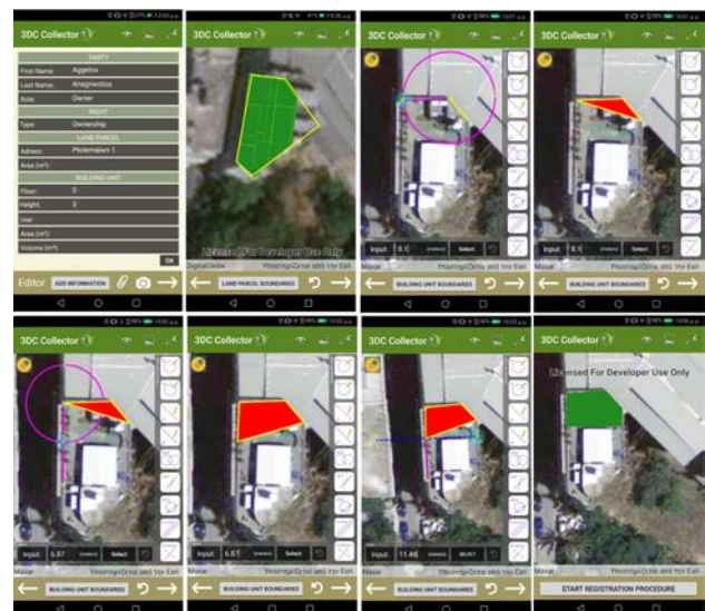
Figure 7. Example of the registration process through the developed mobile application, including (top left) the insertion of the adequate information, (middle top left) the polygon digitization describing the land parcel and (middle top right, top right and bottom) the registration procedure utilizing the geometric tools for the identification/digitization of the polygon describing the building unit, on the basemap
