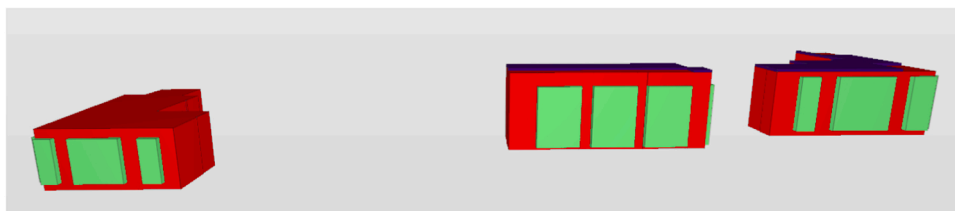
Fig. 13. Three property units of Organellen 100, visualized in Solibri without building elements (Red volumes represent main spaces, green volumes for spaces of windows and blue for spaces of floors).
