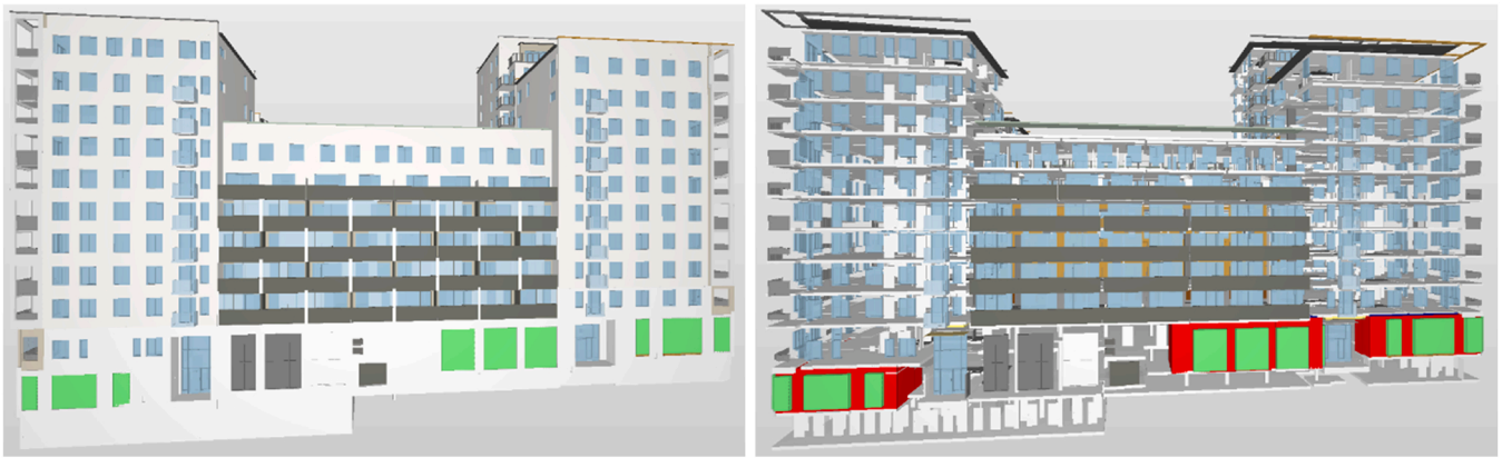
Fig. 14. Left: the property formation model_v1, with created spaces and spaces boundaries for the three property unit areas of Organellen 100. To the right, the model is shown without external walls.
