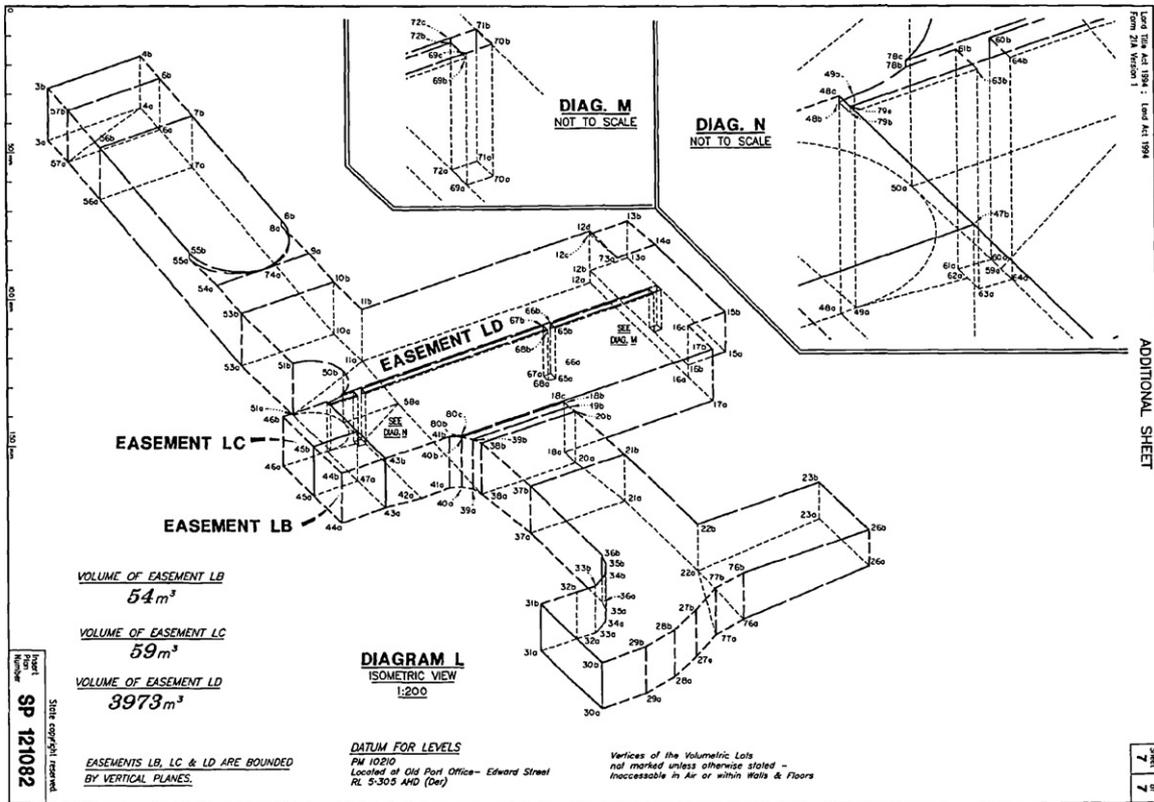
Fig. 13. Example of volumetric survey plan for easement.
