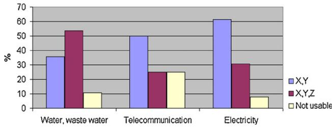
Fig. 5. Coordinate dimension of available utility data.
