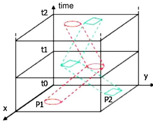
Fig. 4. Representation of two moving objects in integrated treatment of space (2D) and time.
