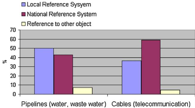
Fig. 6. Spatial reference system of available utility data grouped into pipelines and cables.
