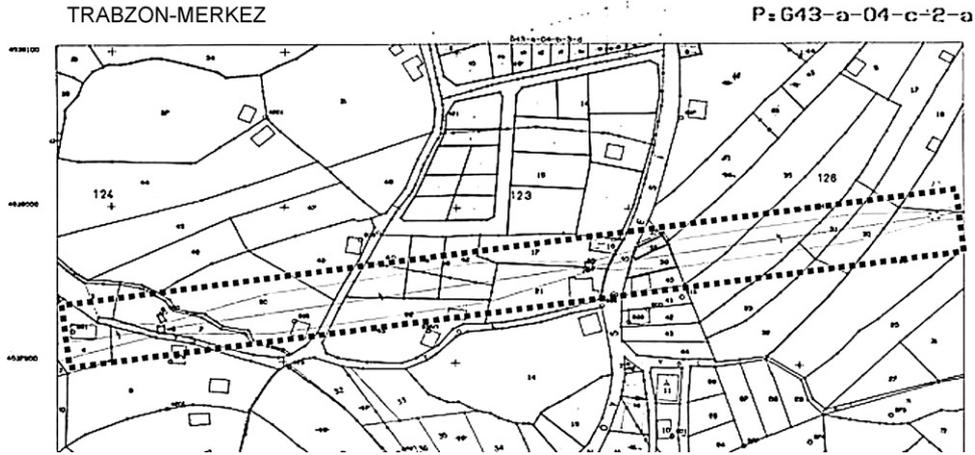
Fig. 8. A cadastre map with high voltage power line (from Demir et al., 2008).
