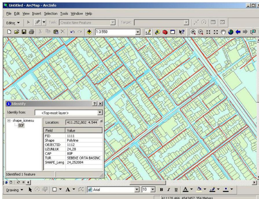
Fig. 7. Network map of gas (red) and water (blue) supply pipelines together with cadastral data. Translation of some of the expressions: 'Uzunluk' = 'length', 'cap' = 'diameter', 'tur' = 'pressure'. (For interpretation of the references to color in this figure legend, the reader is referred to the web version of the article.)
