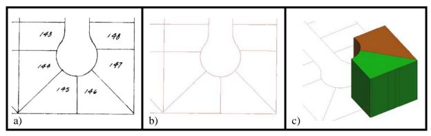
Figure 4. From 2D Raster (a) to 2D Vectors (b) to 3D Solids (c)
