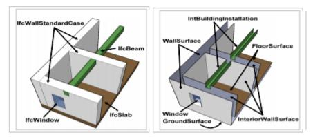
Figure 5. Different modeling paradigm used in IFC and CityGML standards from Nagel et al (2009)
