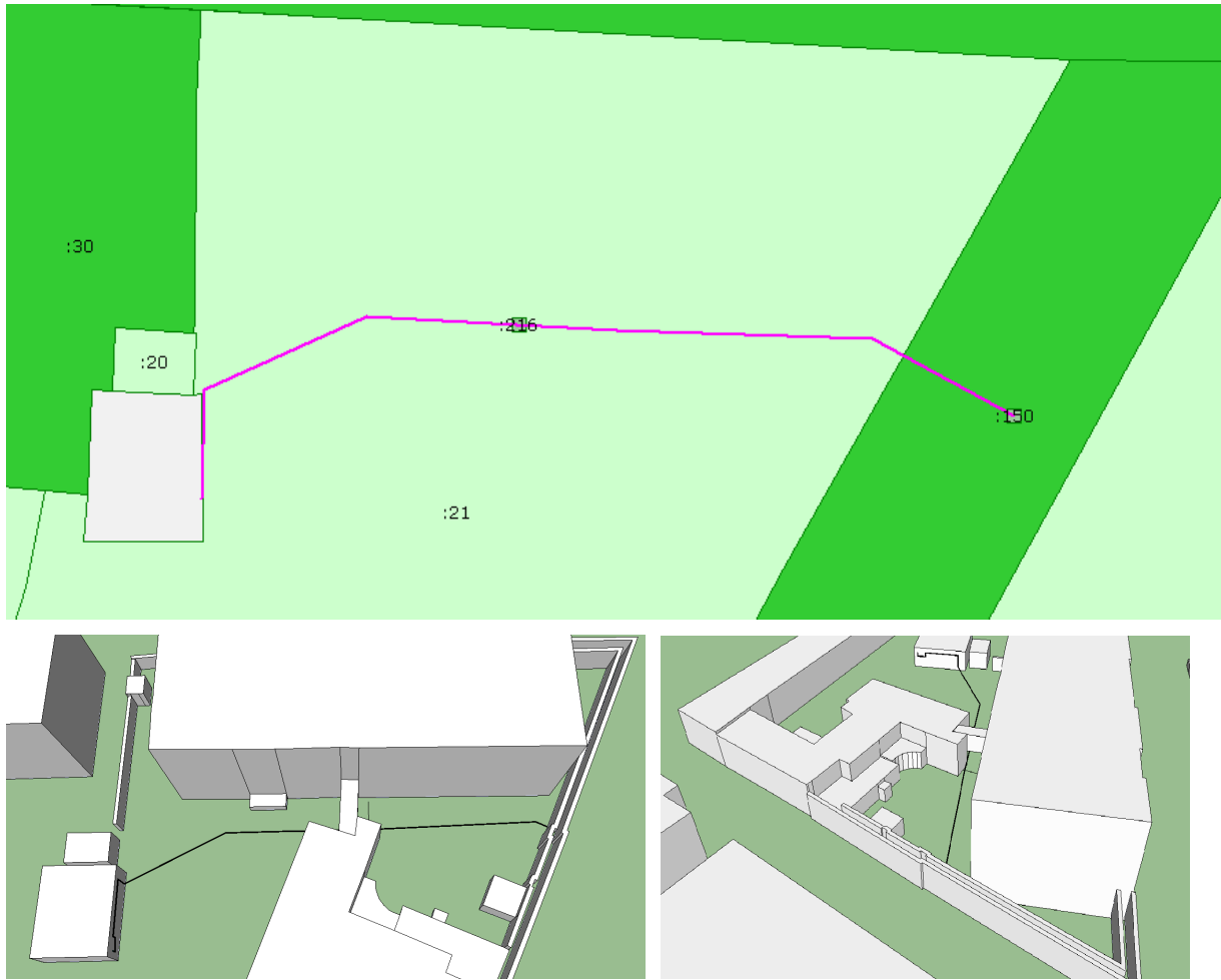
Figure 5. Top: Cadastral map fragment including the pipeline, bottom: two different 3D views
