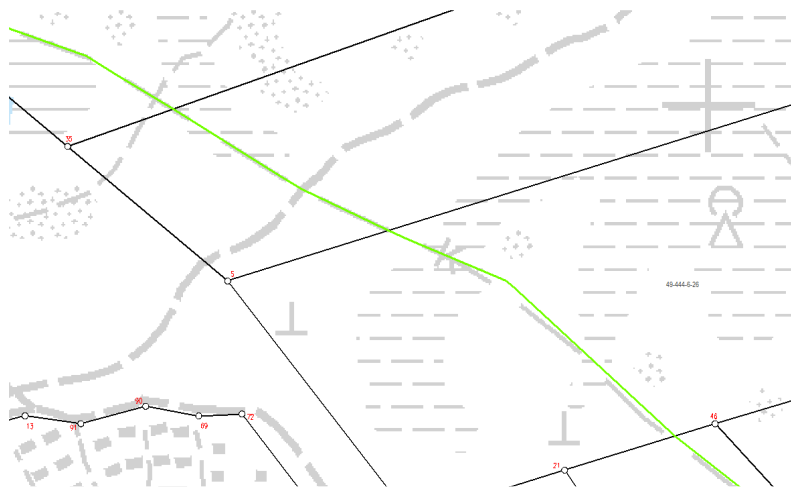
Figure 1. Example from Finland showing gas pipeline in green on the, operational, cadastral map (source http://www.gdmc.nl/3DCadastres/participants/3D_Cadastres_Finland2014.pdf )
