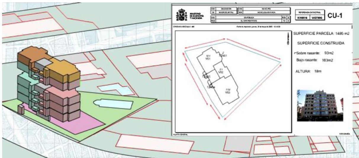
Fig. 2. 3D impression of individual units with floor sketch, photography and relevant attributes (courtesy to the Spanish cadastre) (Doner et al., 2010)
