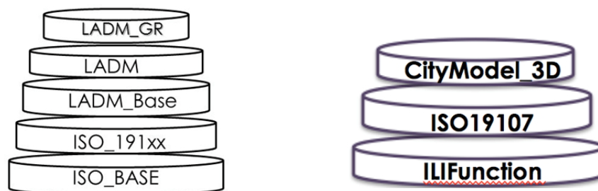
Figure 4a & b. (a) Stack of the INTERLIS models used to describe LADM country profiles (Kalogianni et al 2015): ISO_BASE (basic datatypes), ISO_191xx (geometric primitives and more), LADM_BASE (VersionedObject, Oid), LADM (classes from party, legal, spatial packages), and LADM_GR (Greek country profile), (b) Stack of the INTERLIS models used to describe CityModel_3D: IKIFunction , ISO_19107 and CityModel_3D (Swiss Land Management Group)
