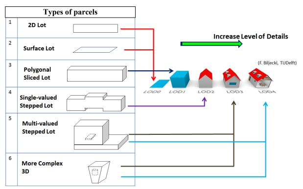
Figure 4. The alignment of different types of parcels with the notion of Level of Details in city modelling
