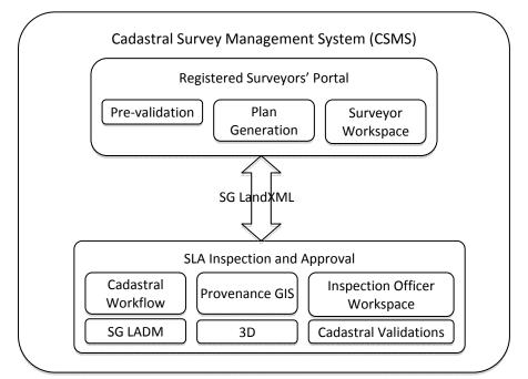
Figure 3. The design architecture of Cadastral Survey Management System, CSMS
