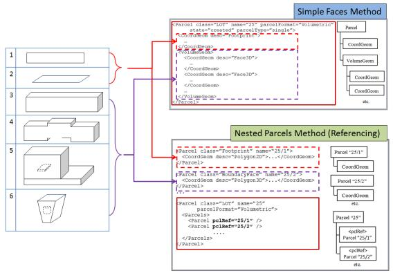
Figure 5. The 6 different types of parcels can be encoded in the simple faces method and the nested parcels method
