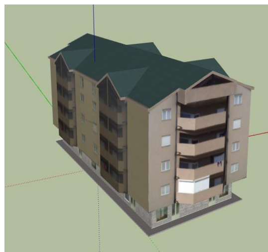
Figure 10. BIM model of a typical building
