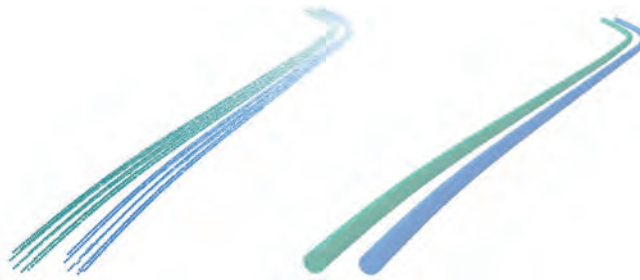
Figure 3: Points in profiles from the laser scanning of tunnels (left) and generated 3D objects representing tunnels (right); Source: with the use of data from "Metro Warszawskie Sp. z o.o."
