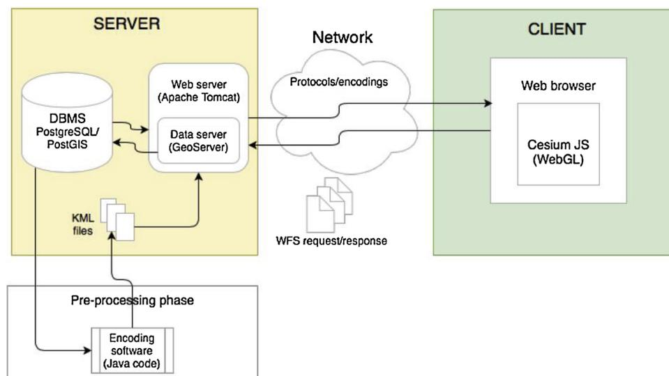
Fig. 4. Server-client system architecture diagram of the 3D cadastre prototype.
