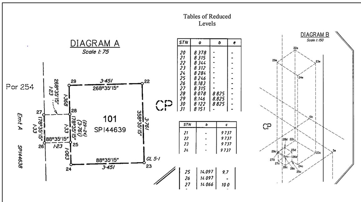
Fig. C1. Excerpts from a Volumetric Plan.
