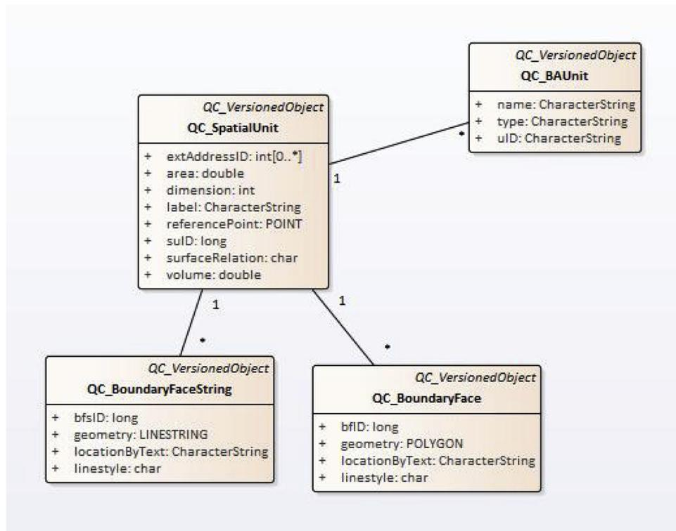
Fig. 8. Spatial Unit structure based on LADM.
