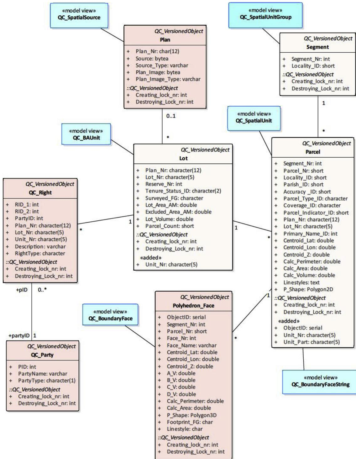
Fig. 9. Database schema of the 3D cadastre prototype. Original tables from the Queensland DCDB are shown in light orange. New tables are shown in red, while the 'views' are in blue.
