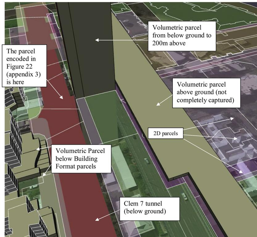
Fig. 6. A mixture of 2D parcels, Building format and Volumetric parcels.
