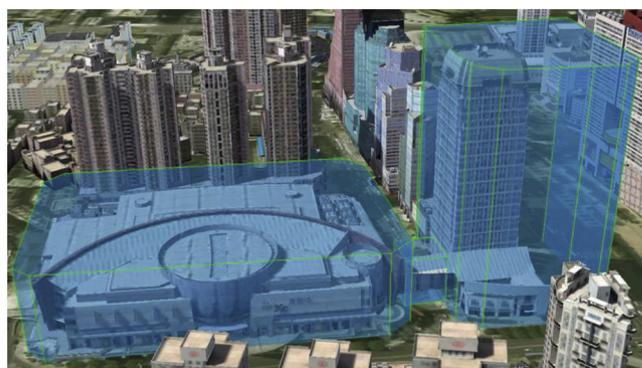
Fig. 1. Use of transparency to enhance the difference between physical and legal objects (Ying et al. 2012).
