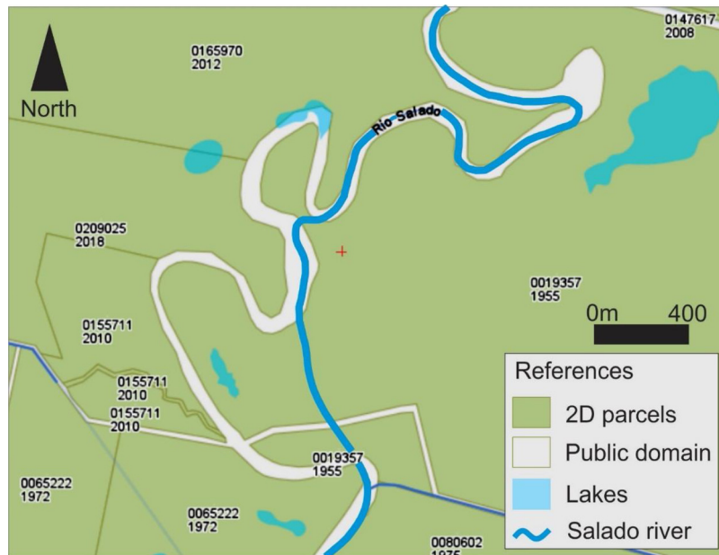
Fig. 2. Cadastral inconsistencies between parcel limits and digitized channels. Source: Cadastre and Territorial Information Service, Santa Fe, Argentina.
