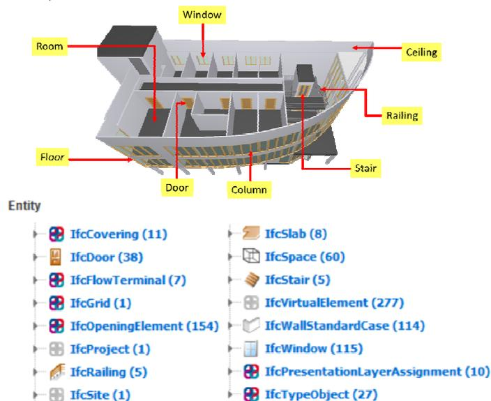
**Figure 2: The IFC model for 3D cadastral purpose.**
