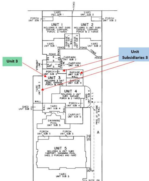
**Figure 10. Floor plan diagram for a Strata Plan**
