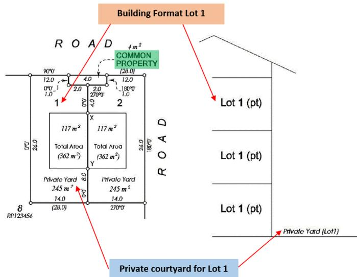
**Figure 7, Examples for building format plans
