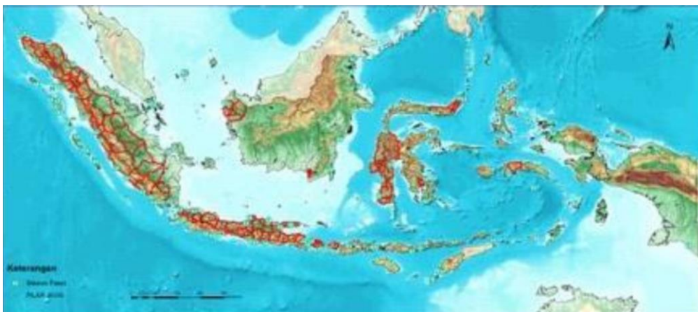
Fig. 2. Distribution of the vertical ground survey marks (source: https://srgi.big.go.id )
