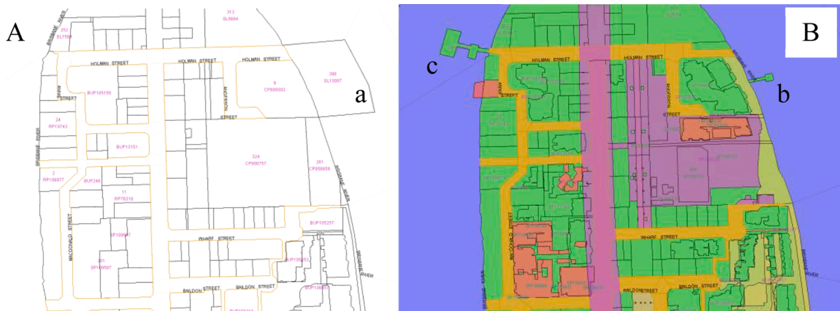
Fig. 5. A: Queensland Cadastre in 2001. B: Queensland Cadastre in 2013 (from Thompson, 2015). Broad changes can be seen in the cadastre in Fig. 5 – parcel a (extending into the river) has been replaced by a more closely defined jetty structure b; jetty c has been captured, and many volumetric (purple) and strata (red) spatial units have been captured.
