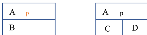
Fig. 3. Topology Preservation: Where a spatial unit B is subdivided, a point representation p is created, although in fact, the real-world point has always existed along the boundary between A and B. A finite representation of p, however will almost certainly not lie on the line, and the introduction of p will cause a slight bend.
