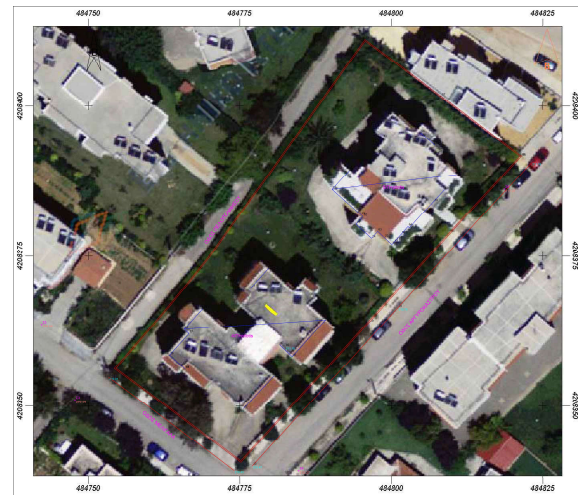
Figure 13. An orthophoto overlaid with the topographic diagram derived from the field surveys
