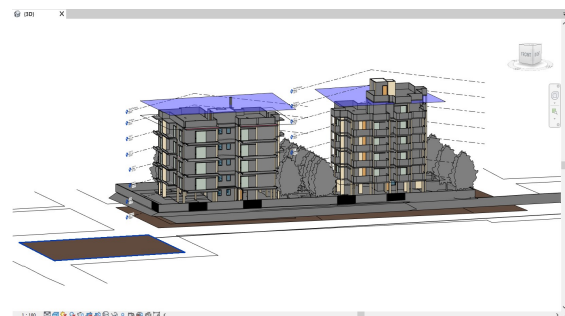
Figure 20. Height and development restrictions, as 3D surfaces
