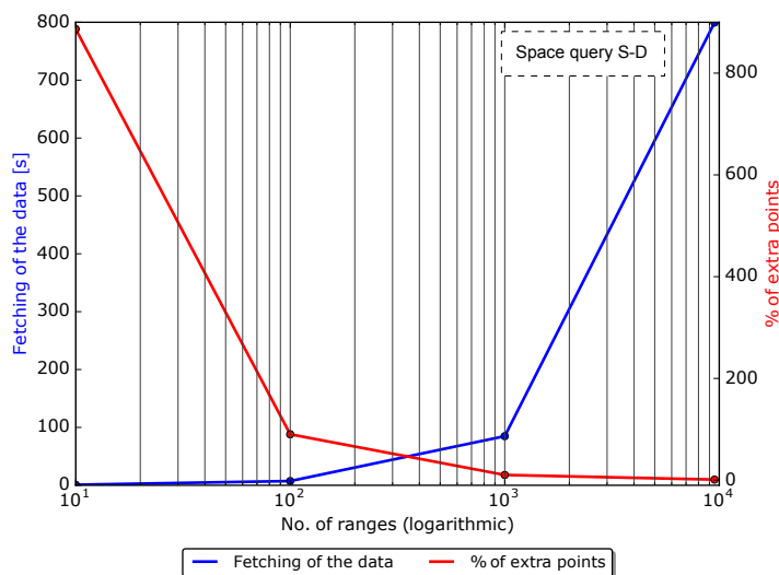
Figure 5.9: Effect of imposing a different degree of merging in the same original Tree Cells on the percentage of extra points obtained and the fetching time. Case: Space only queries in the non-integrated approach (treatment of z as an attribute). S-D represents line with buffer of 5 metres (11933 points).
