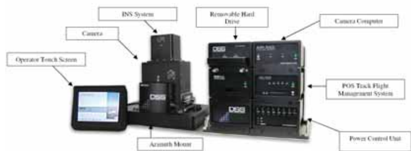
Figure 1 Configuration of the Applanix Digital Sensor System DSS
