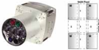
Figure 5 The UltraCamX sensor head (left) consists of eight camera heads, four equipped with 9 CCD sensors in their four focal planes and contributing to the large-format panchromatic image. The focal plane of the Master Cone carries four CCDs (right).
