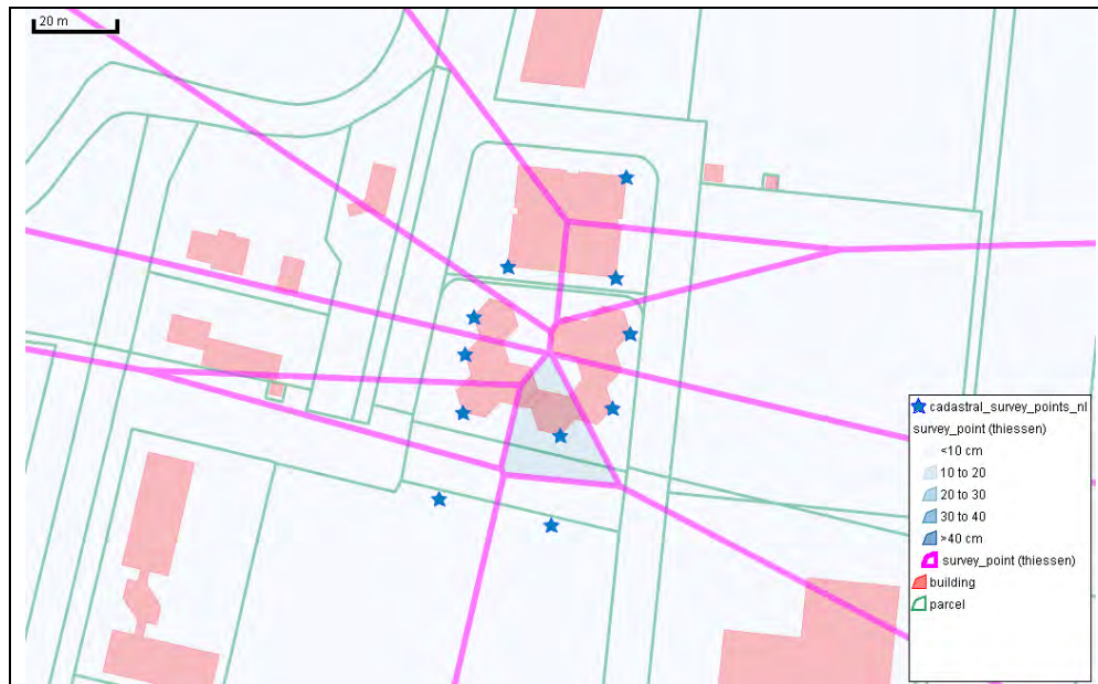
Figure 67 - Connection Points overlaid with Thiessen Polygons
