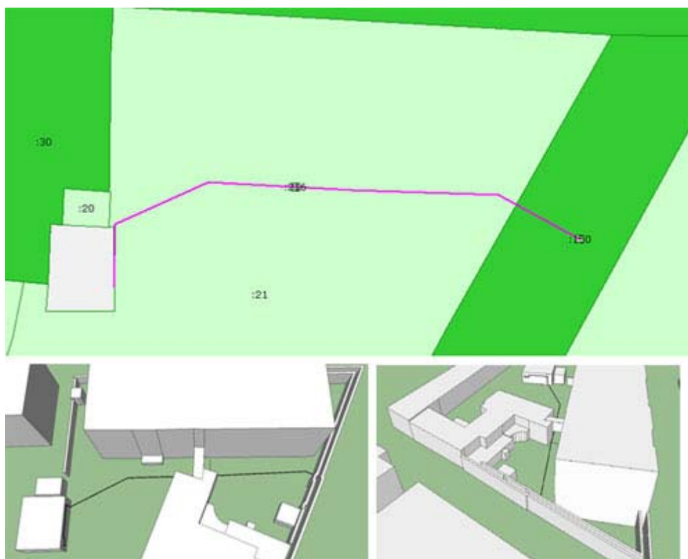
Figure 3. Top: Cadastral map fragment including the pipeline, bottom: two different 3D views
