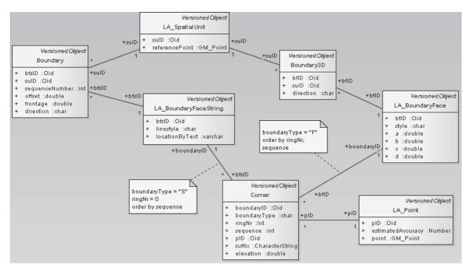
Fig. 7. Suggested data model, based on proof of concept database piloted using the Queensland DCDB data.
