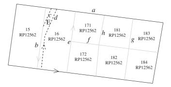
**Fig. 12.** Generic encoding – note that in contrast with earlier figures, lower case letters are used to label face-strings rather than individual line segments. For example, '*a*' refers to the outer (road) boundary starting and ending at the top left corner.
