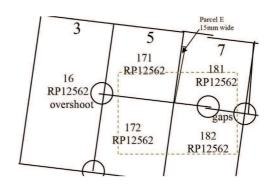
**Fig. 5.** The arrowed small parcel is similar in size to the gaps and overlaps in the data. Any automated cleansing will cause it to be lost or corrupted.
