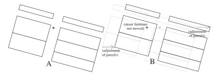
**Fig. 1.** (A) Positioning street furniture in relation to cadastre. (B) Where the positioning of the parcels is adjusted due to an improved survey, the position of the street furniture must also be changed to maintain relativity.
