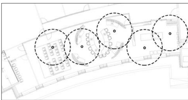
Figure 3: Range of the individual receivers on the floor, based on the conical angle
