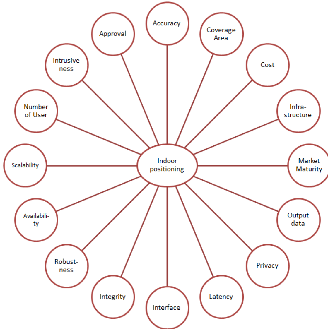
Figure 5.5: Indoor positioning performance factors (Mautz, 2012)
