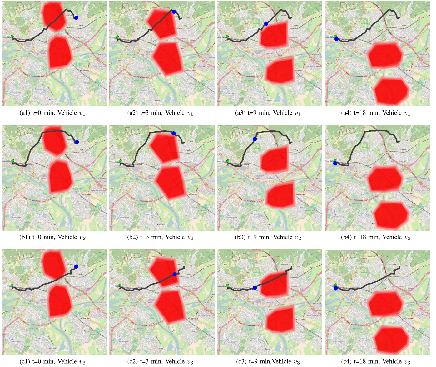
Fig. 14. Snapshots of routes calculated for 3 vehicles (in blue circle) with different r_{max} . The vehicles have the same source and destination points. The shapes and positions of the obstacles (in polygons) are the same in the three simulations, and change as the vehicles are moving towards the destinations. (a) Vehicle v_1 , r_{max} = 0 min. (b) Vehicle v_2 , r_{max} = 2 min. (c) Vehicle v_3 , r_{max} = 7 min.
