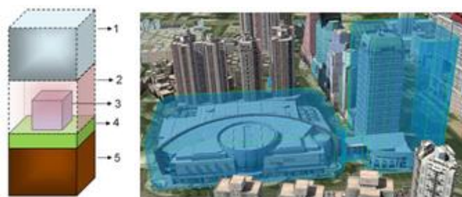
Figure 21: (left) The "layer" approach to the 3D cadastre (Source: Dimopoulou and Elia, 2012), (right) The structures visible in blue - the legal space of the 3D cadastral parcel. Space of construction in the form of a 3D city model (inside the legal space). Source: Ying et al. (2012)
