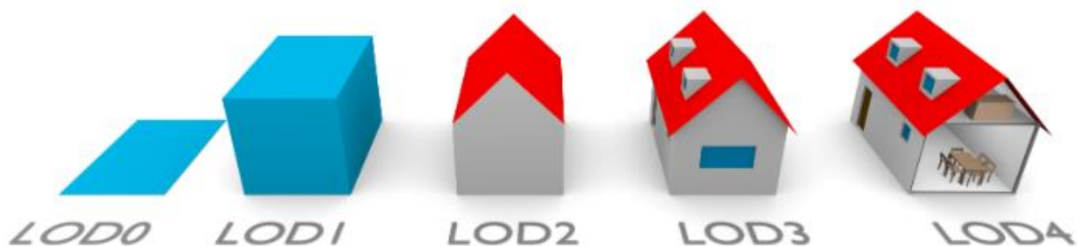
Figure 2. The five LODs of CityGML 2.0. The geometric detail and semantic complexity increase, ending with LOD4 containing indoor features (Biljecki et al., 2016)
