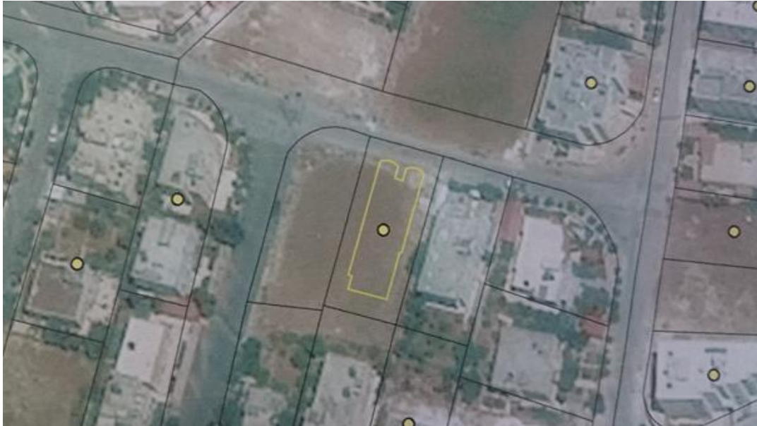
Figure 19: Example from the cadastral map database with a new building footprint (yellow polygon) and the Department of Lands and Survey building coordinate (yellow dot). Aerial photo is used as background. (Courtesy of the Department of Lands and Survey, Amman, Jordan)
