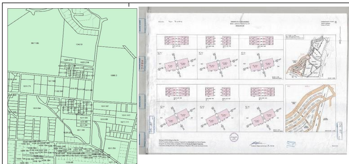
Fig. 10. Trinidad and Tobago's digital 2D cadastre Fig.11 Vertical sections on survey plans depict 3D rights
