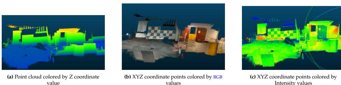
Figure 1.5: Three modalities of a point cloud
