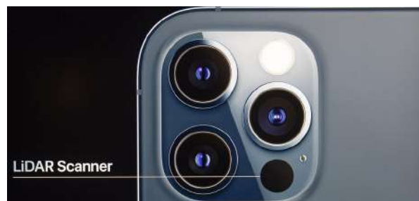
Figure 8.6: Back side of the Apple iPhone 12 Pro Max, showing its 3 camera lenses and the LiDAR scanner; Daniel Acker/Bloomberg, from this Forbes article
