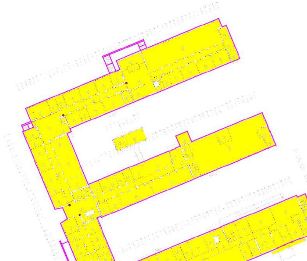
Figure 8.7: Part of the ground floor floor plan, in the process of being digitized. The thin red lines represent interior rooms, and are marked on the original floor plans. The thick purple lines are polylines (added in QGIS) used to represent exterior boundaries of the building.
