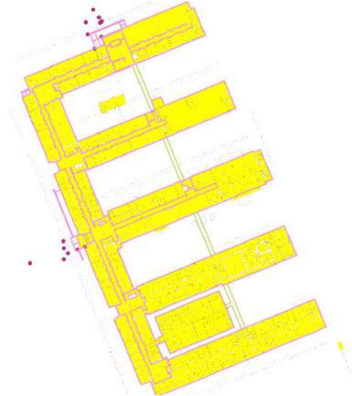
(b) The ground floor exterior and interior walls are now digitized, in pink. The brown-yellow lines represent the glass walkways present on the first floor of the building.
