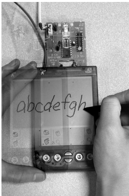
Figure 3.30 Example of peephole method to write text longer than the screen by moving both hands co-ordinately whilst writing
